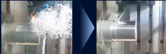
Comparison of results between regular turning operations and CBS II machining
